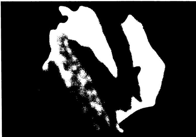
FIG. 4. Backscattered electron image of a 15- \mu m pentlandite grain in Maralinga. The variable contrast indicates considerable compositional heterogeneity and suggests a mixture of two phases.
